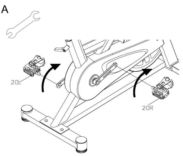
Screw R/L pedals (20) onto crank (18). The pedals are marked with R and L at the screw. Tighten the left pedal counter-clockwise, the right pedal clockwise.
