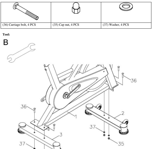
While another person lifts the front of Frame (1), attach the Front stabilizer (2) to the Frame with two M10x55mm Carriage bolts (36) from the above Stabilizer, and fix it with two 10x19x1.5mm Washers (37) & two M10 Cap nuts (35).
