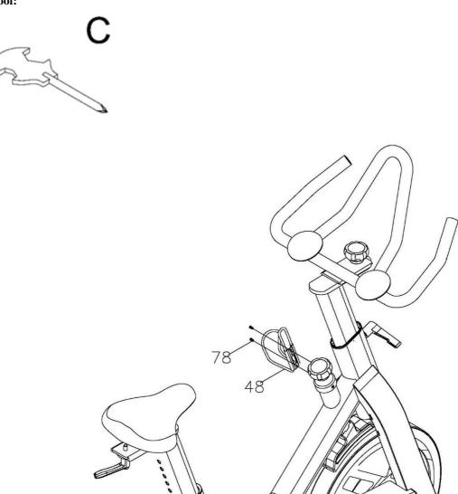
Release two M5x15mm Bolts (78) from the Frame (1), then put the Bottle holder (48) onto the Frame (1) and relock two Bolts (78).
