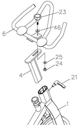
Release the Spring knob (21), then insert the Upright post (4) into the Frame (1). There are 5 holes on the Upright post (4), please select the desired position and tighten the Spring knob (21). Next connect the Handlebar (6) with the Upright post (4), select the desired position and fix it with one M10x28mm Knob (23), one 10x29x2mm Washer (46), one 19.5x38x2mm Washer (25) and M10 Lock nut (24).
