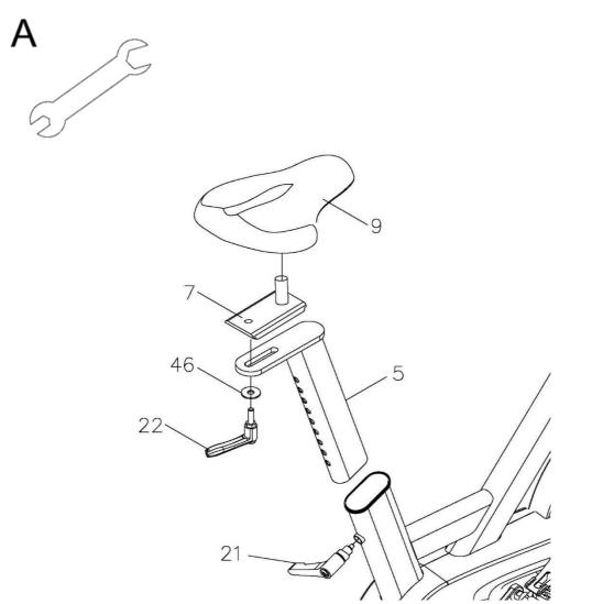
Release the Spring knob (21), then insert the Seat post (5) into the Frame (1). There are 9 holes on the Seat post (5), please select the desired position and tighten the Spring knob (21). Next attach the Seat (9) to the Moving bracket (7), then connect the Moving bracket (7) with the Seat post (5), select the desired position and fix it with one M10 L-knob (22) & one 10x29x2 mm Washer (46).
