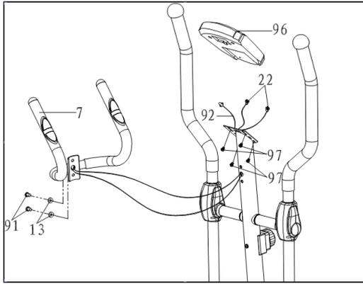
Remove four M5x12 Bolts (97) from the back of the Computer (96). Remove bolts with the Multi Hex Tool with Phillips Screwdriver provided.
