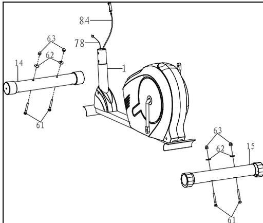
Position the Front Stabilizer (14) in front of Main Frame (1) and align bolt holes. Attach the Front Stabilizer (14) onto the front curve of the Main Frame (1) with two M8x70 Bolts (61), two Ø8xØ25 Big Curve Washers (62), and two M8 Cap Nuts (63).
