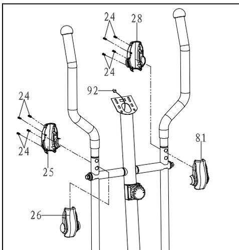
Attach the Left Handrail Arm Cover-A (25) and Left Handrail Arm Cover-B (26) onto the Left Handrail Arm (3) with four ST2.9x12 Screws (24). Tighten screws with the Multi Hex Tool with Phillips Screwdriver provided.
