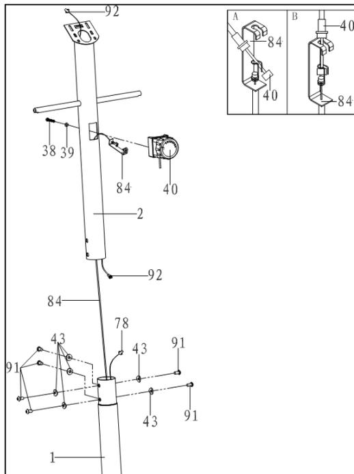
Remove six M8x15 Bolts (91), six Ø20xØ8x2.0 Big Curve Washers (43), from the Main Frame (1). Remove bolts and washers with the S6 Allen Wrench provided.
