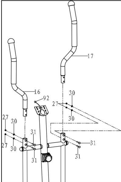
Attach the Left/Right Handrails (16, 17) onto the Left/Right Handrail Arms (3, 4) with four M6x35 Bolts (31), four Ø6xØ12x1 Curve Washers (30), and four M6 Cap Nuts (27). Tighten cap nuts with the Multi Hex Tool with Phillips Screwdriver provided.
