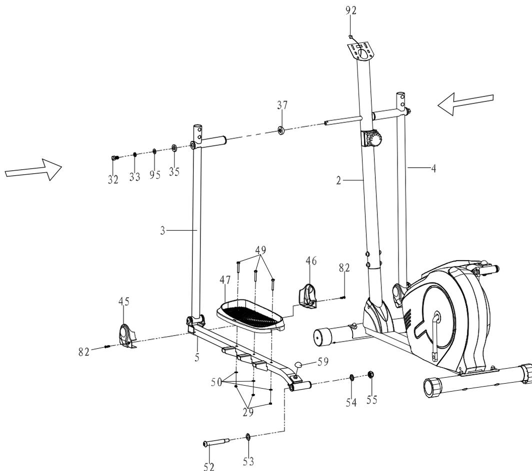
Remove two M10x18 Bolts (32), two Ø10 Spring Washers (33), two Ø10xØ20x2.0 Big Washers (95), and two Ø28x5 Washers (35) from the left and right horizontal axes of the Front Post (2).
