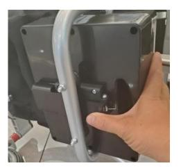
Grasp the battery and pull it out of the frame.
