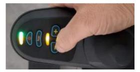
Press the horn, the controls will switch to pairing mode.
