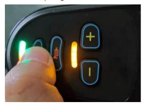
Hold down the down arrow on the remote control until the power button on the remote control stops flashing.
