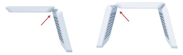
Connect the side panels to the top panel (control panel)
