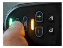
Press the power button on the remote controller for 5 seconds.
