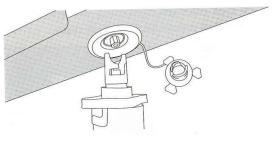
6. Connect the air tube to the valve.
