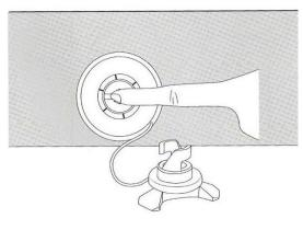
5. Press the valve and turn it counterclockwise by 45 degree.
