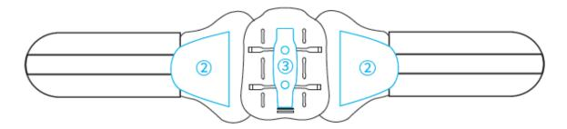
You can adjust the panels (2) with Velcro and hooks. The middle plate (3) is removable.
