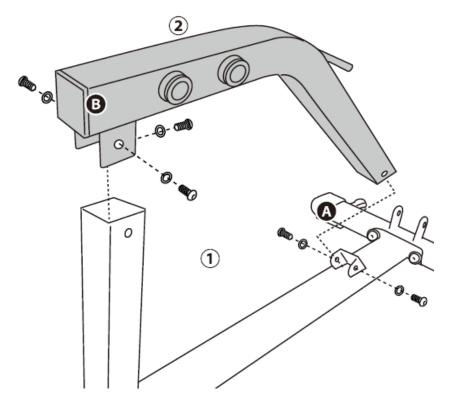
Remove the bolt, axle and washer from the saddle bracket (4) and secure the saddle bracket (4) to the bent frame (2) with the bolt, axle and washer removed.
