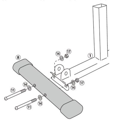
Attach the stabilizer (7) to the main frame (1) with 2x bolts (11), 4x washers (14) and 2x nuts (17).
